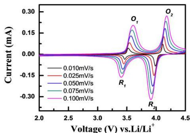
5 CV curves of  $\text{LiFe}_{0.4}\text{Mn}_{0.6}\text{PO}_4/\text{C}$  annealed at 600°C
