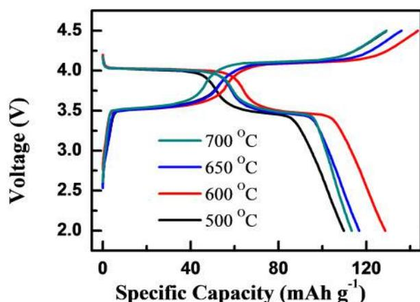
4 Initial charge–discharge profiles at 0.1 C
