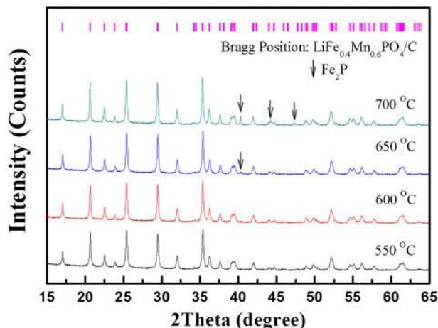
1 XRD patterns of  $\text{LiFe}_{0.4}\text{Mn}_{0.6}\text{PO}_4/\text{C}$  composites synthesised at different temperatures
