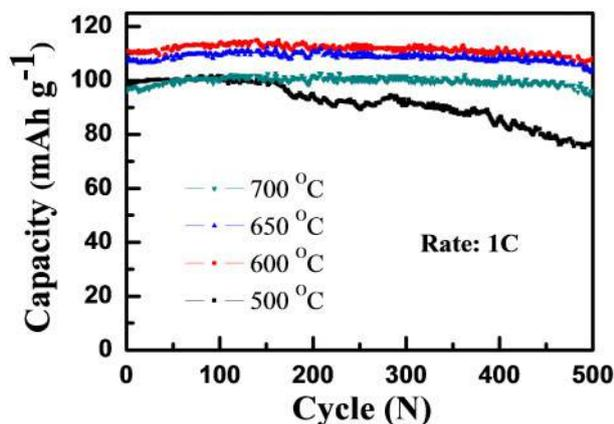
6 Cycle performance at 1 C of  $\text{LiFe}_{0.4}\text{Mn}_{0.6}\text{PO}_4/\text{C}$  composites synthesised at different sintering temperatures
