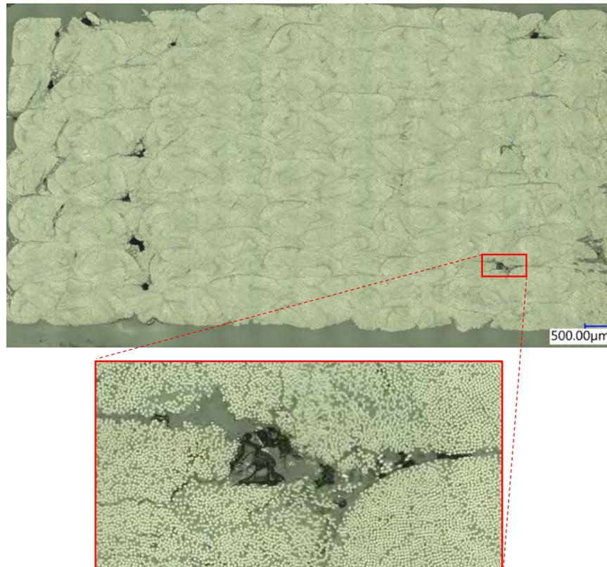
Figure 6.4: An example test image (top image: 18,270\*10,306 pixels), the details of the fiber cross-section distributions and resin-rich areas can be better observed by zooming in on local regions (bottom image).
